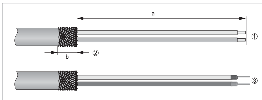
Figure 4-15: Preparation of field current cable C
