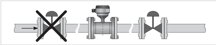
Figure 3-10: Installation in front of a control valve
