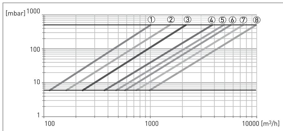
Figure 6-5: Pressure loss between 1...9 m/s / 3.3...30 ft/s for DN200...600 / 8...24"
