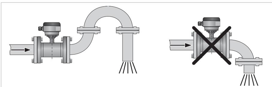
Figure 3-6: Installation in front of an open discharge
