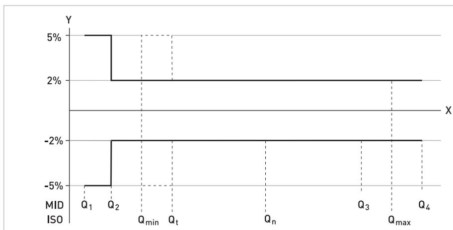
Figure 6-2: ISO flow rates added to figure as comparison towards MID
