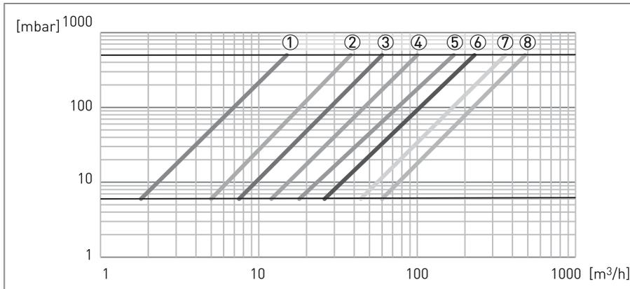
Figure 6-4: Pressure loss between 1...9 m/s / 3.3...30 ft/s for DN25...150 / 1...6"
