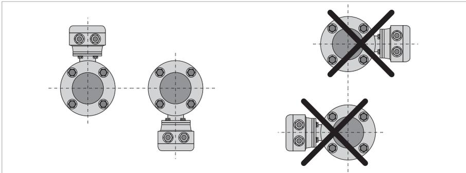
Figure 3-13: Mounting position
