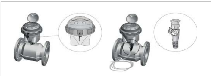
Metrological seals on the compact version and cable connection
