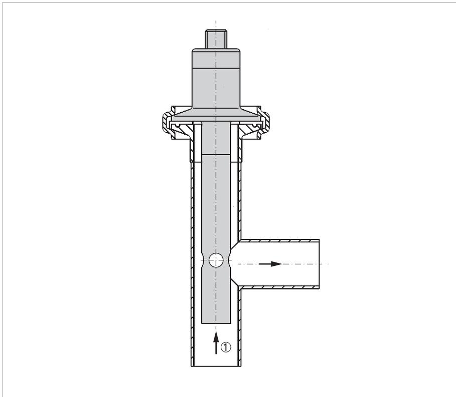
Figure 3-1: Mounting position
