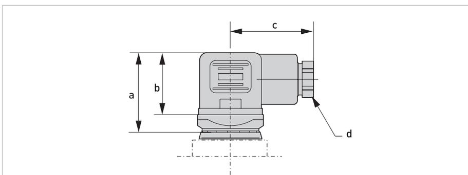
Figure 2-2: Angled connector (Hirschmann)
