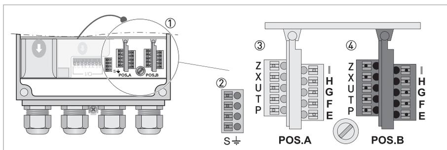
Figure 4-3: Junction of the signal converter
