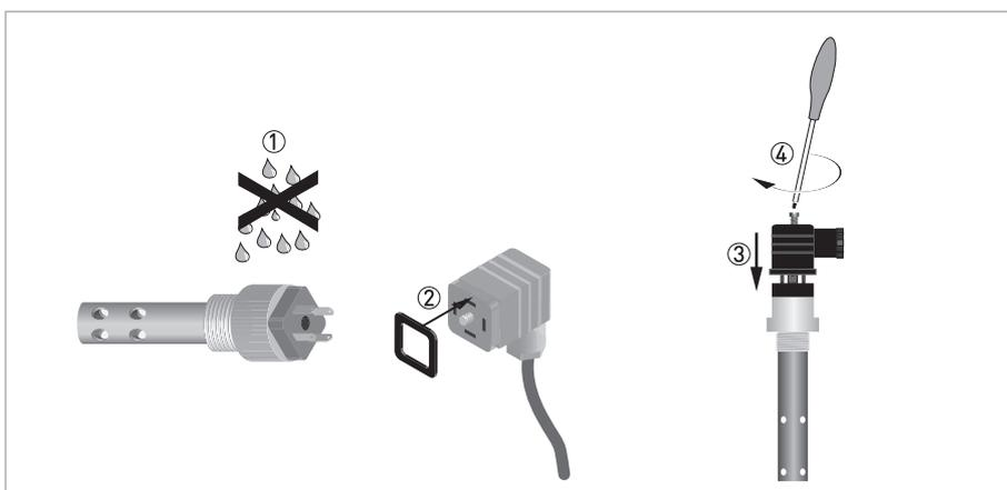
**Figure 4-1: Connecting the Hirschmann plug to the sensor**
