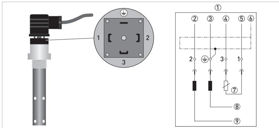
Figure 4-2: Cable assign of a Hirschmann plug
