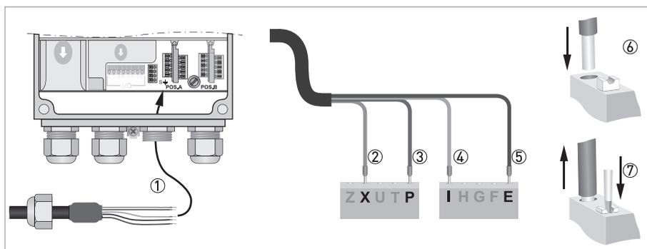
Figure 4-4: Connecting the sensor cable to the signal converter
