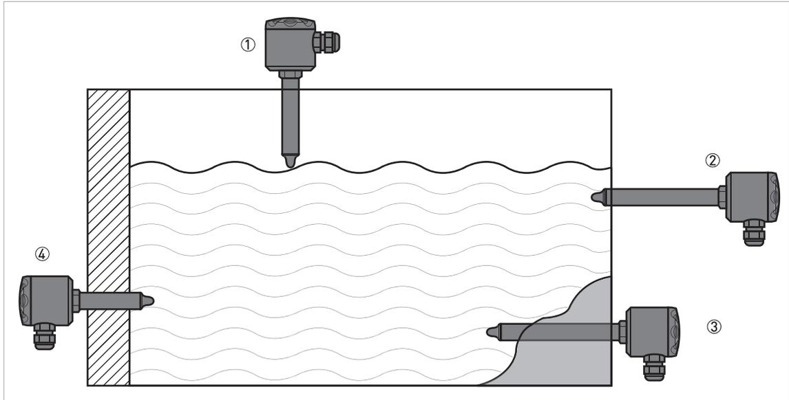
**Figure 3-1: Possible applications for sliding connection**
