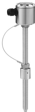
The OPTISWITCH 6500 C is in two longer versions (100 mm and 250 mm / 3.9" and 9.8") available. The device is installed with a special packing gland adapter which allows a flexible insertion length. The devices can be used on high-temperature applications up to +200°C / +392°F; the stem is then working as a cooling neck. Alternatively, the device can be installed with this option on tanks and pipes with insulation or on level applications with a lower switching point level.
