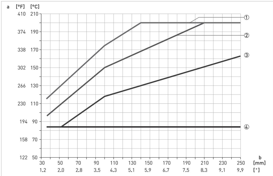
Figure 3-2: Media temperature against external length of sliding connection
