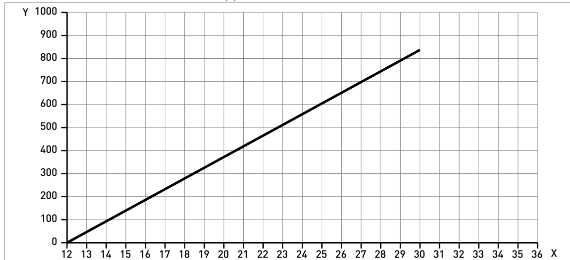
Figure 2-3: Minimum power supply voltage for an output of 21.5 mA at the terminals (Non-Ex and Hazardous Location approval (Ex i / IS))
