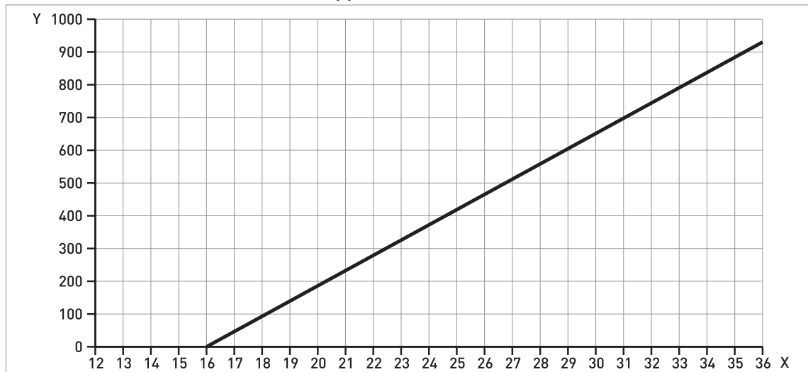
Figure 2-4: Minimum power supply voltage for an output of 21.5 mA at the terminals (Hazardous Location approval [Ex d / XP/NI])
