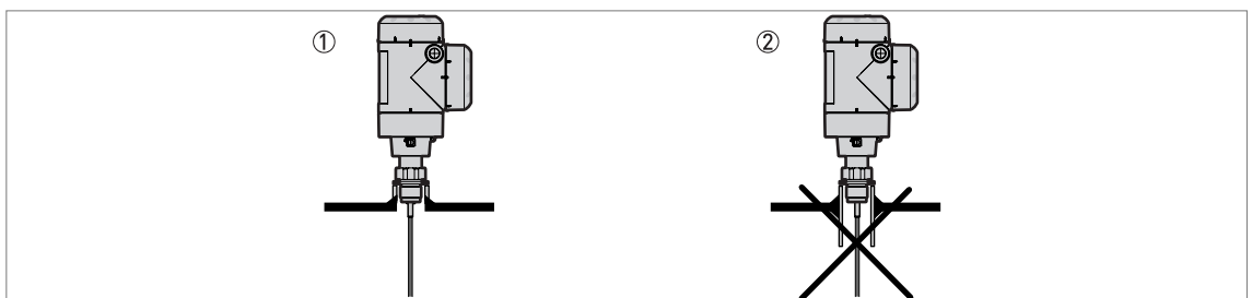
Figure 3-4: Sockets for threaded process connections
