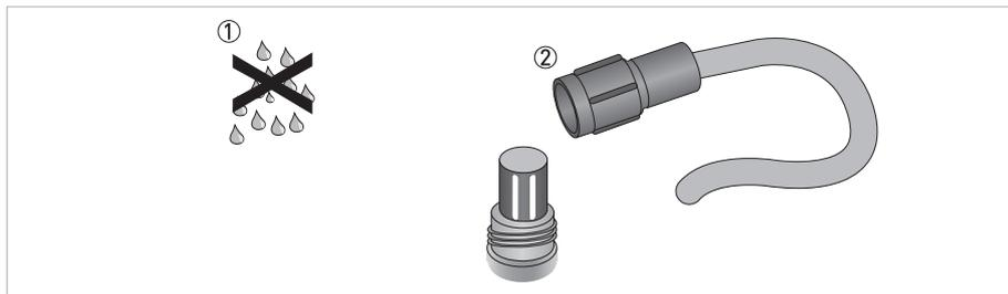
Figure 4-1: Connecting the cable to the sensor
