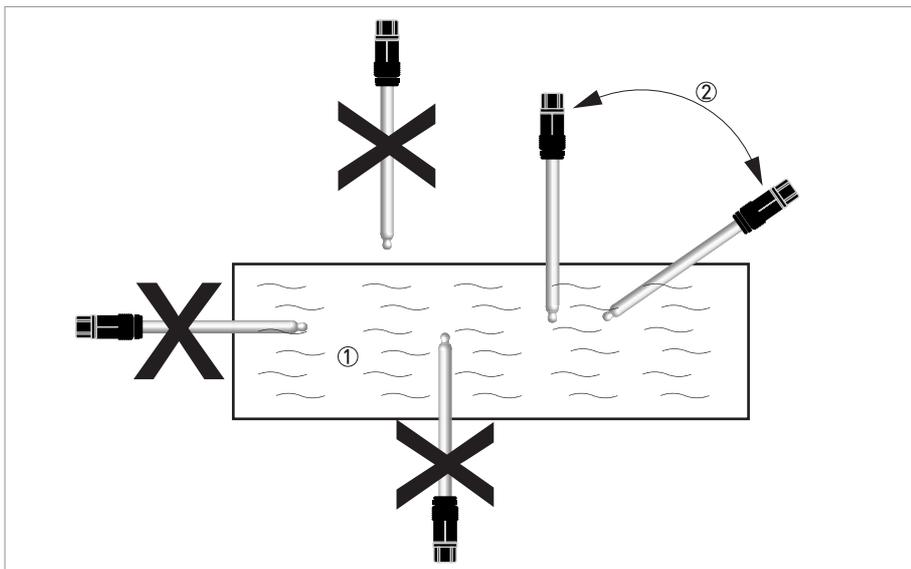
Figure 3-2: Installation requirements
