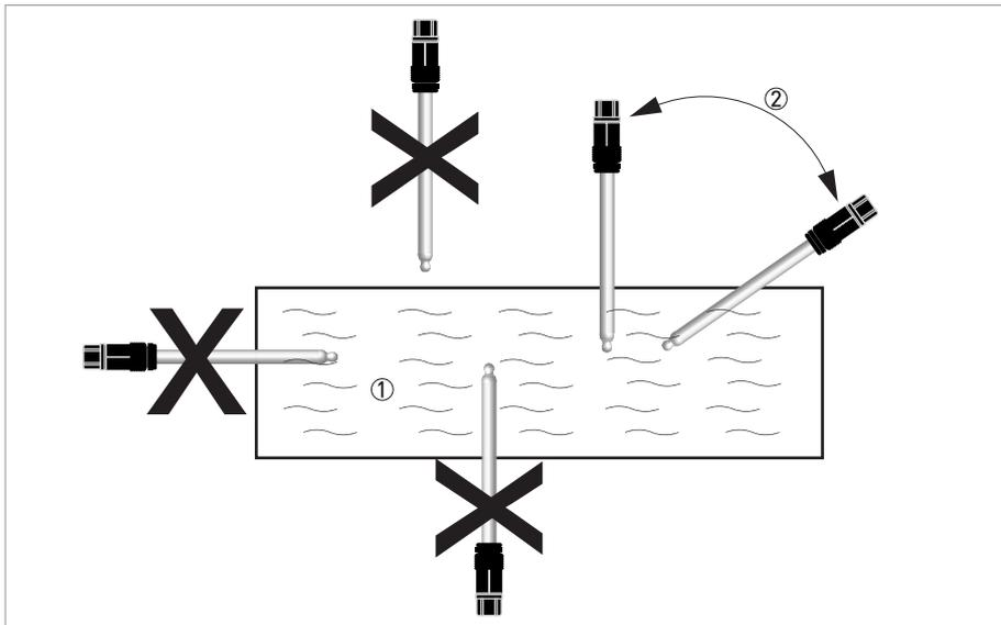
Figure 3-2: Installation requirements
