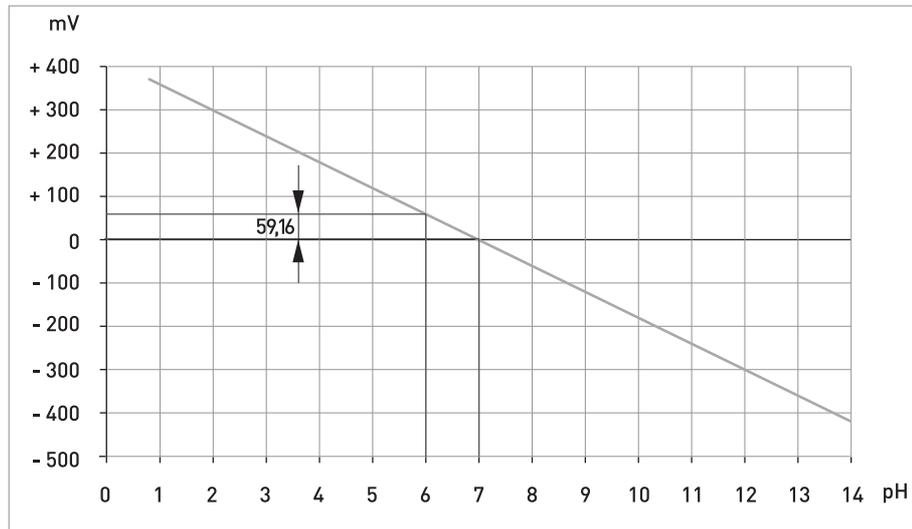
Figure 1-2: Optimal slope at 25°C / 77°F
