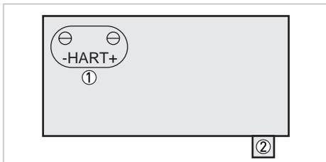
Figure 4-3: Example of a HART® handheld connection
